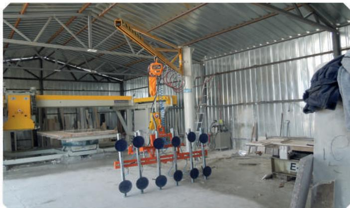
Vakumer is manufactured for lifting big pieces of marble, granite and travertine plates or strips with vacuum technology. The system works with vacuum pump or ejection. Vakumer 500 Can be mounted on a Jib Crane or X-Y bridge Crane. The turning system is optional such as pneumatic, hydraulic or mechanic.
